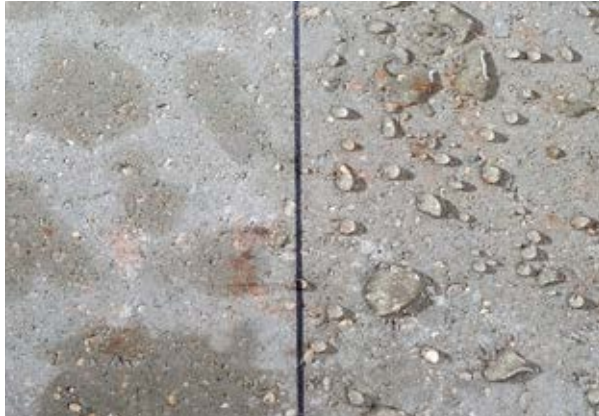
Untreated concrete (left) versus concrete treated with Salt Protector Plus™ WB (right).
